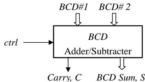
Figure 2 A BCD adder/subtractor to be designed.
