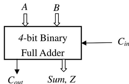
Figure 3 A 4-bit binary full adder.
